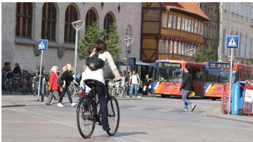
Cyclists and buses, but not cars, share the area around this bus terminal. It works since the speed limit is low. Aalborg.
